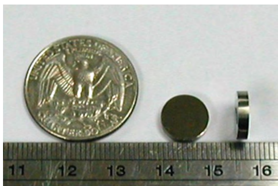
Fig. 4. The outer morphology of the \text{Ti}_{50}\text{Cu}_{28}\text{Ni}_{15}\text{Sn}_7 with 4 vol.% CNT addition after vacuum hot pressing at 723 K under a pressure of 1.2 GPa.
